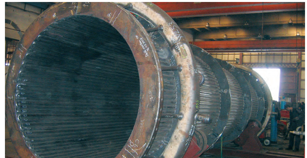
Offgas duct during manufacturing
