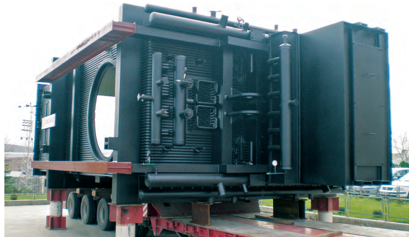
Drop out box for offgas section behind EAF
